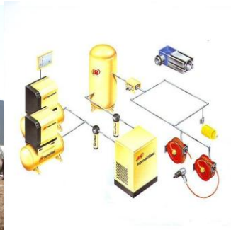
Station Air Comprimé
